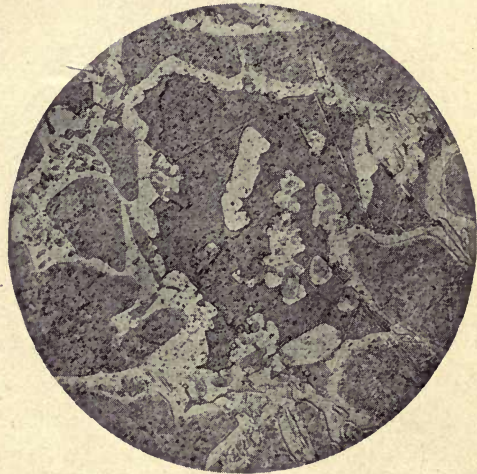
Fig. 14. Alloy D. Cu 78.0 Annealed at 565° C. Sn 22.0 For 3 hours and quenched.
